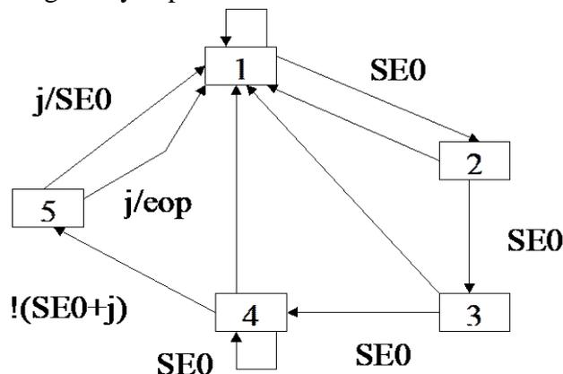
Fig 1 EOP detection state machine
