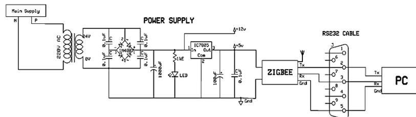
Figure 2. Circuit Diagram of Smart Robot (receiver section)
