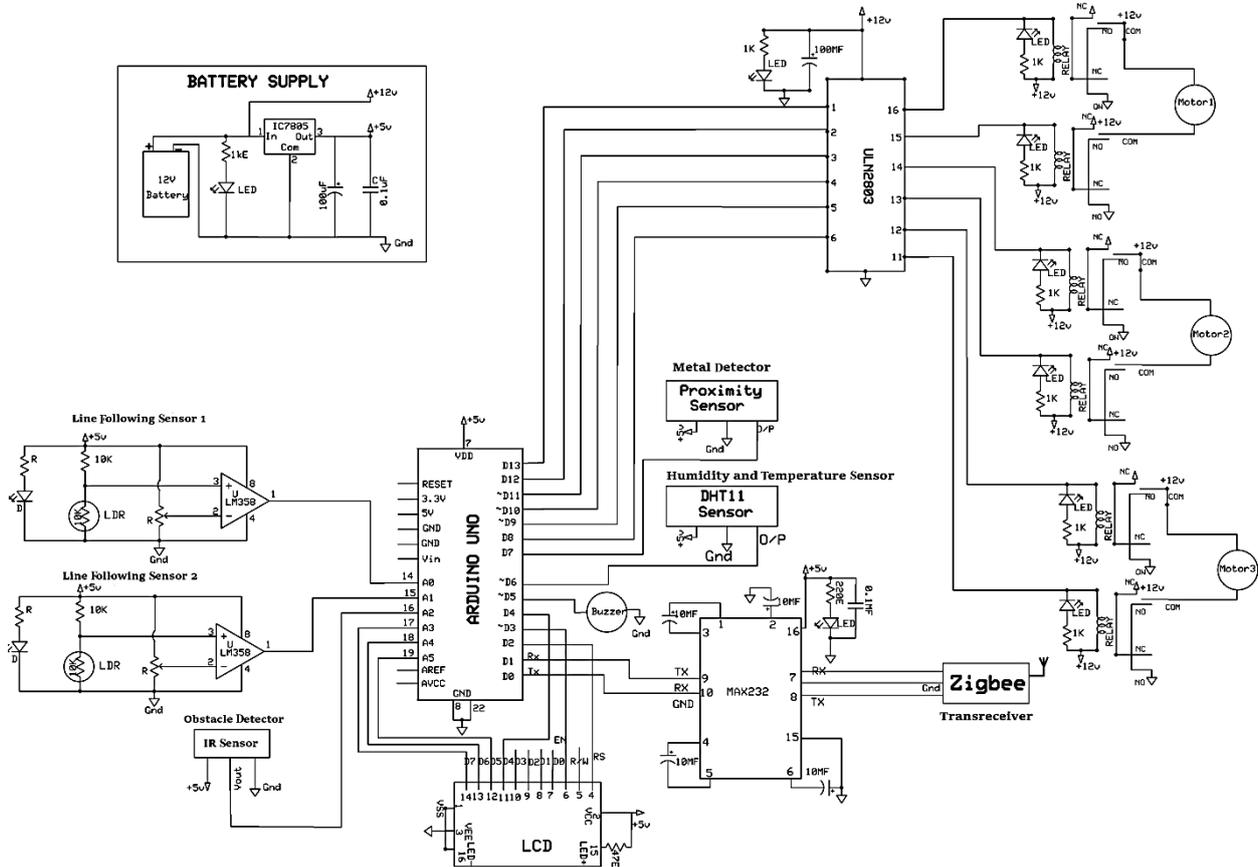
Figure 1. Circuit Diagram of Smart Robot (transmitter section)
