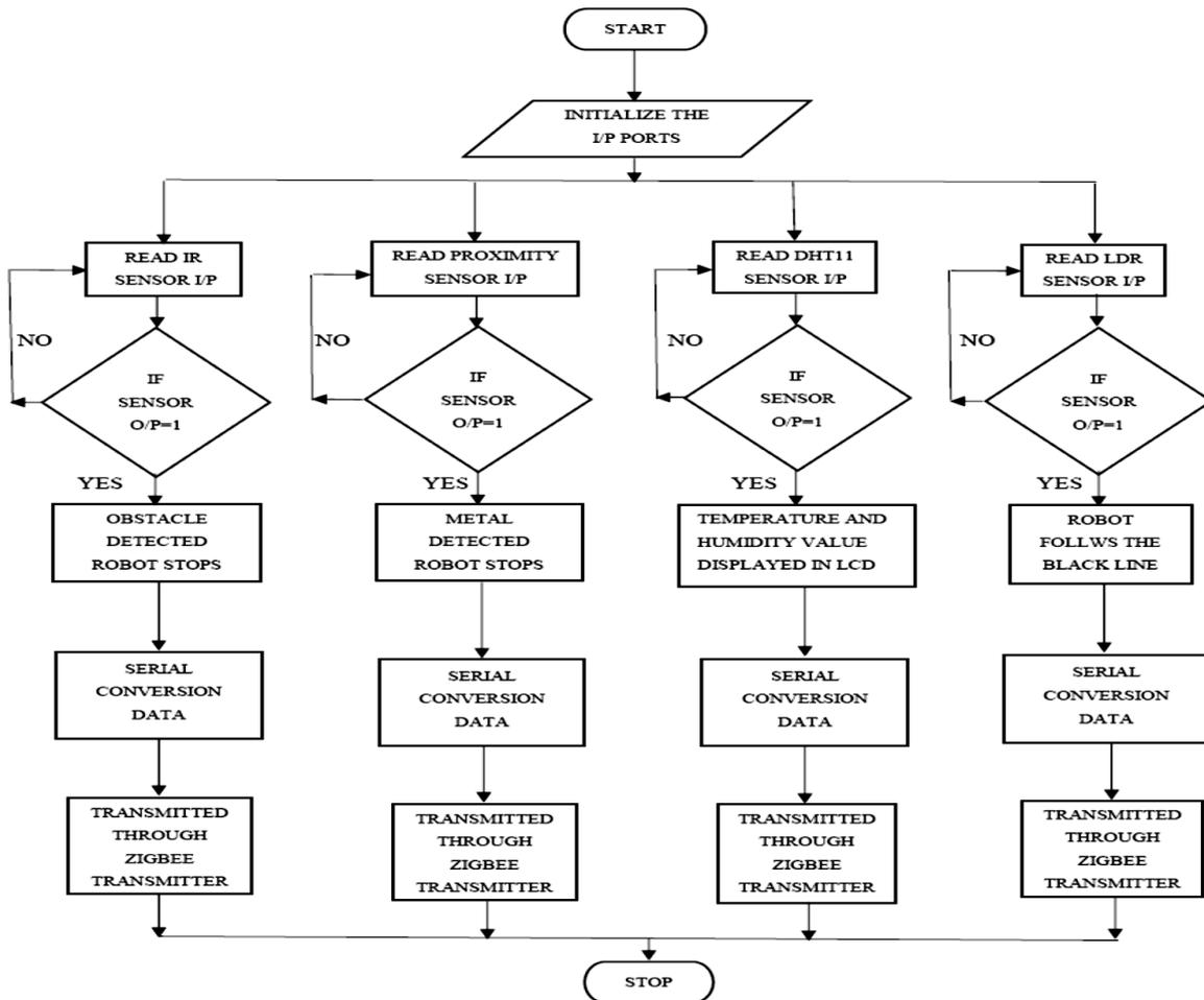
Figure 3. Flow chart of Smart Robot (transmitter section)
