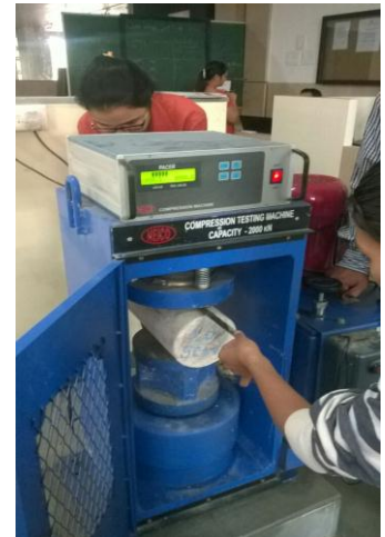
“Figure4.Spliting Tensile Strength Test set up”
